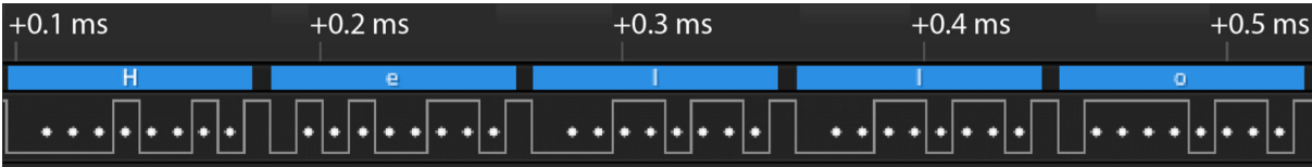
Figure 7.3 – Screenshot of the logic analyzer tool showing the first 5 bytes sent by the example to the host using UART3
