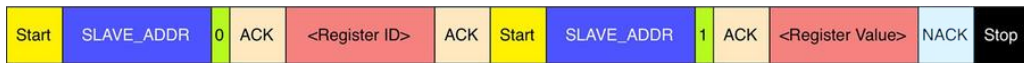
Figure 12: The I 2 C protocol used to read internal register of our slave device
