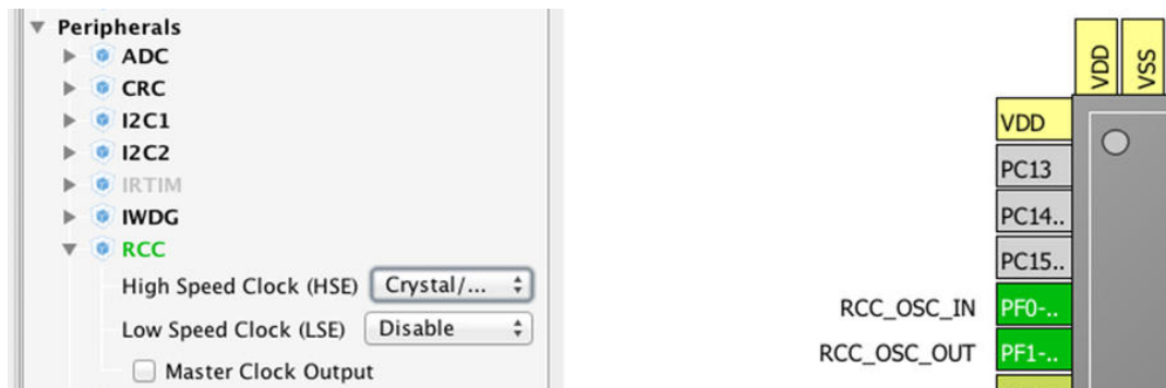
Figure 6: The configuration options provided by the RCC peripheral
