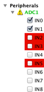
Figure 11: The IP Tree view pane allows to select input channels of the ADC
