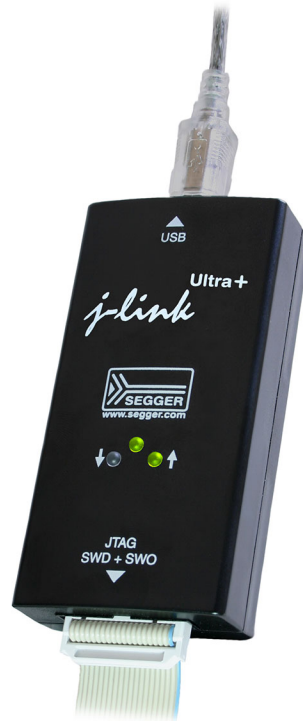
Figure 19: A SEGGER J-Link Ultra+ debug probe
