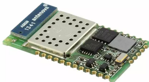
Figure 1: The SPWF01SA WiFi monolithic module
